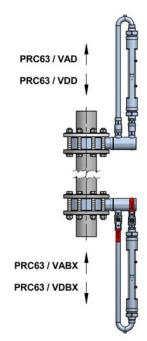
ED: flow from left to right DES: flow from right to left DAB: downwards flow BD: upwards flow
