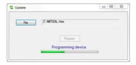
The process takes about 90 seconds, after which the message "Device programmed" will appear.
