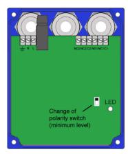
With the switch in the **maximum** level position, the common contacts of the relays are in "normally open" when the detector is not in contact with the liquid/solid (level below the detector), and change to "normally closed" when the detector is submerged. The LED changes from green to red.
