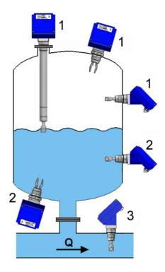
In positions 1 the LD6XR acts as a maximum level switch. In positions 2 the LD6XR acts as a minimum level switch and in position 3 it acts as a liquid presence detector (for example, to protect a pump).
