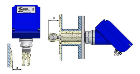
If the filling of the tank is above the level where the LD6XR must be installed, try to move the detector away as much as possible, and If during the filling of the tank strong waves are produced, the level detector must be protected.
