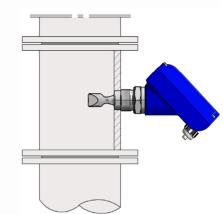
If the viscosity is high, the flaps must be kept away from other objects (such as the wall of the tank or a nozzle).
