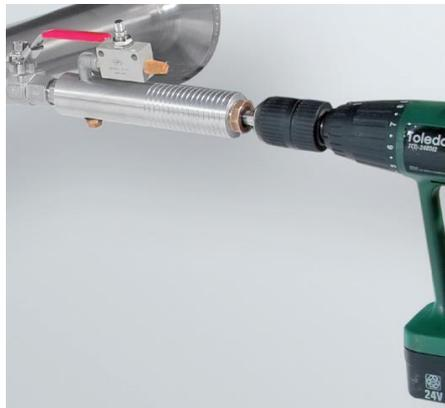
In case the system could not be shut down, means to be set depressurized, there could be used the CS spot drilling collar and drilling jig to drill through the ball valve.
